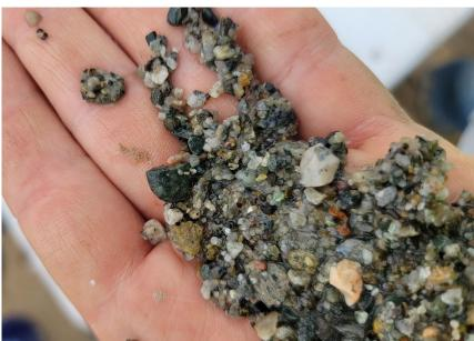
Photo 7. Drill cuttings from aquifer zone. Note the coarse and medium-grained sand particles.
